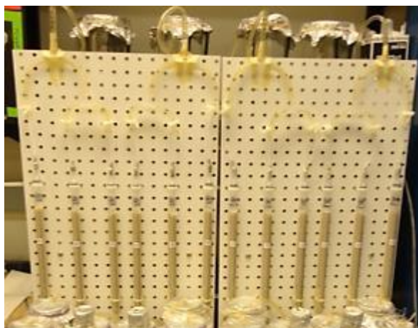
Figure 2. The first trial SSF bioreactor design which contained 12 bioreactors. Fountain pump jars were located on the shelf behind a pegboard used to secure the tubing system and the sand syringes.
