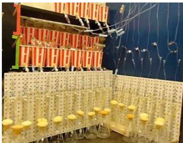
Figure 3. The second trial SSF bioreactor design which contained 20 new bioreactors. IV bags were held upright in red popcorn tubs above a pegboard used to secure the IV lines and the sand syringes.
