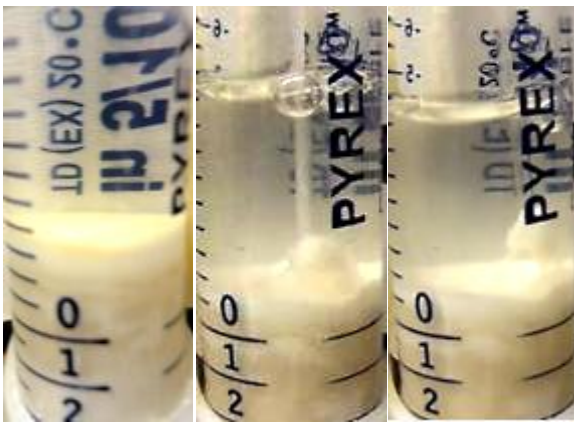
Figure 5. After the experiment concluded, probing the cake layers revealed that there was a pink or white elastic pudding-like substance mixed in with the sand.
