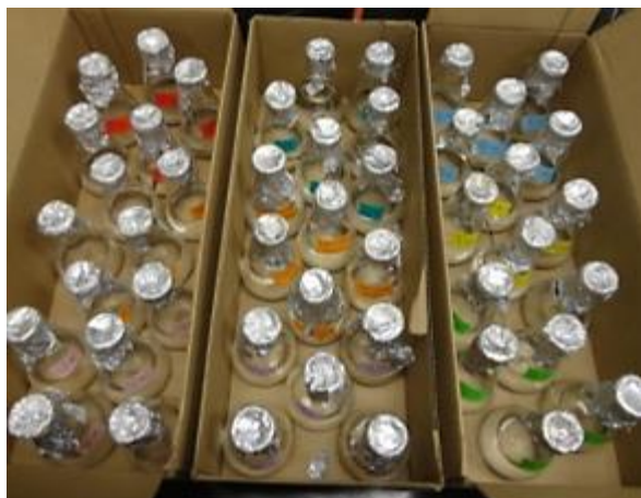
Figure 1. The 45 PBC bioreactors built during the isolate selection process. Three replicates of each of the seven bacterial isolates as well as sterile controls were created and monitored.
